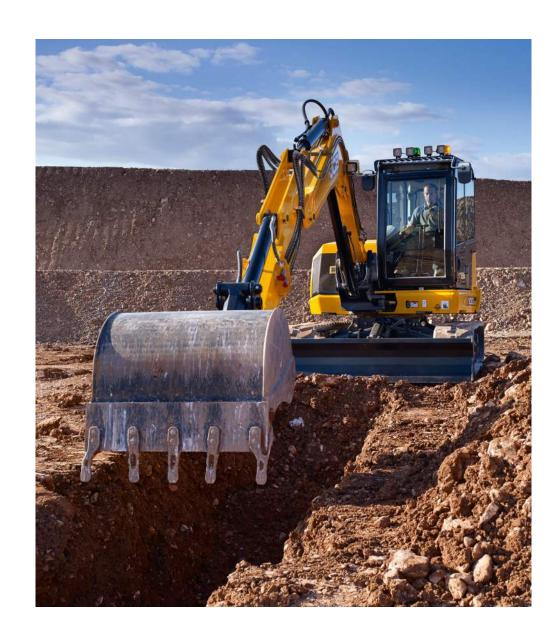
The fully compliant ROPS and TOPS\* cab has excellent front visibility courtesy of a 70/30 front screen split. It also provides a clear view of the front right track for easy, safe trench digging and manoeuvring. Overall, we have improved overhead visibility from the cab making truck loading easier and safer.
