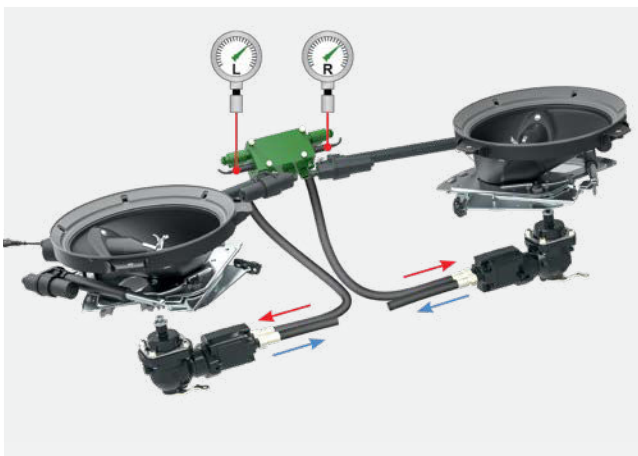
✔ FlowCheck sensors in the hydraulic circuit
