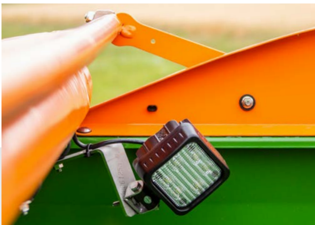
Lighting for the inside of the hopper
