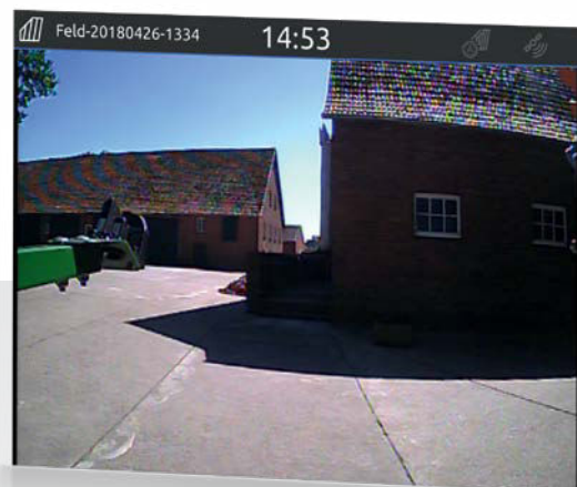
Display of the camera image in AmaTron 4
