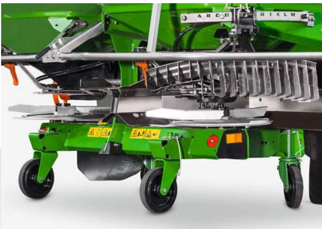
Special frame with rolling and parking device
