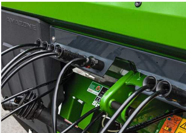
Accessible holder for the hydraulic hoses
