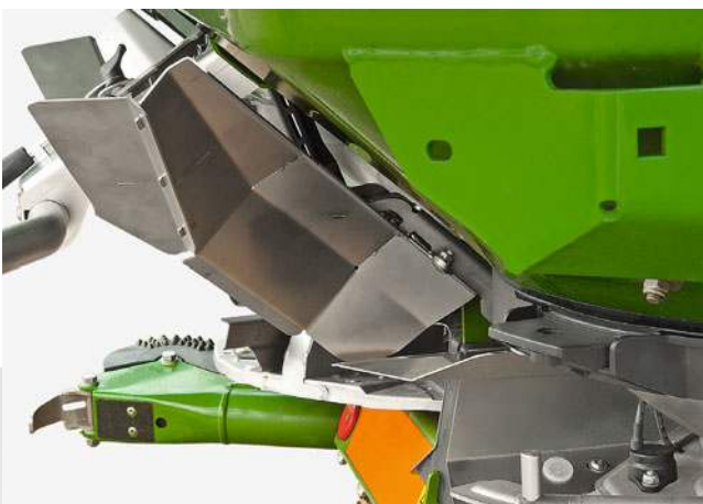
Border spread deflector folded upwards
