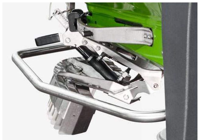
Limiter V hydraulic border spreading system
